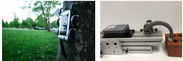
Fig. 1: The T-RHex robot hanging from a tree (left), and the testbed used for comparing leg designs equipped with a single T-RHex leg (right).
